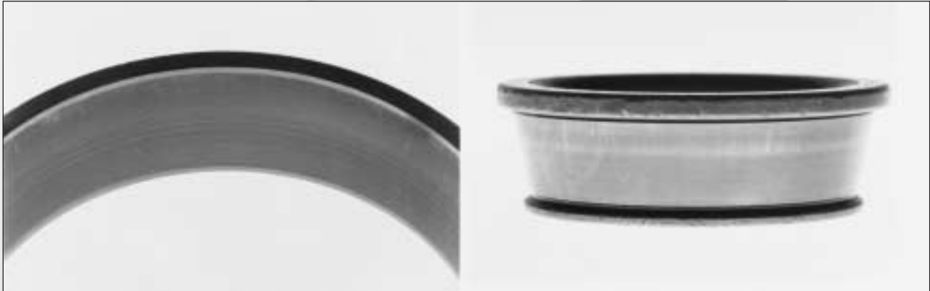
Abrasive wear. Usure abrasive. Abrieb.
