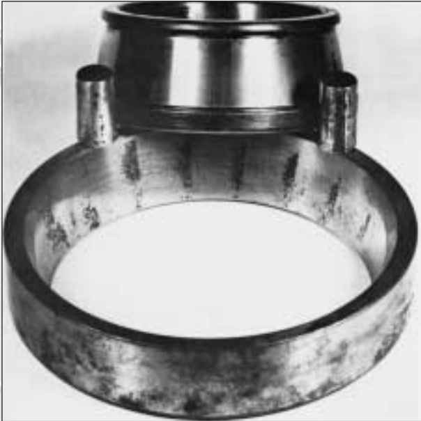
Etching in the initial stage Pitting caused by moisture at the roller/raceway contact line.
